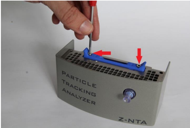
Figure 14-6: Fix the screws tightly. Do not overtight them.
