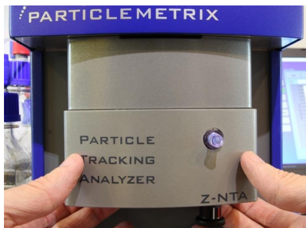
Figure 4-2: Push the Cell assembly carefully using both hands. Do not apply force while pushing it towards the front of the ZetaView® instrument.
