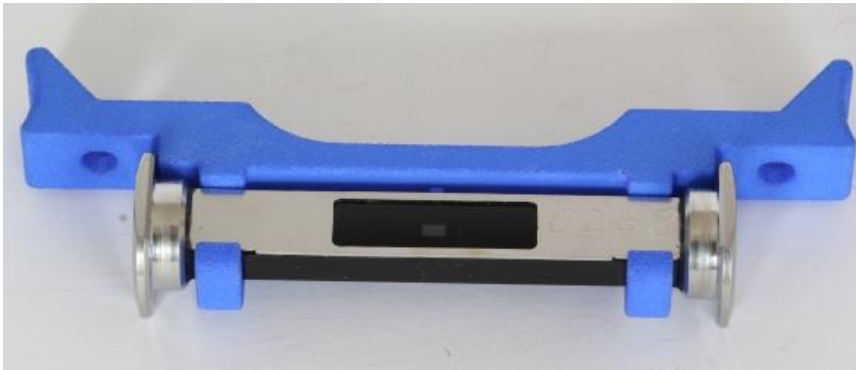
Figure 4-14: Cell and cell carrier are attached to each other. Please note that the cell is attached such that the serial number is still visible at the open part of the cell carrier's right bracket.
