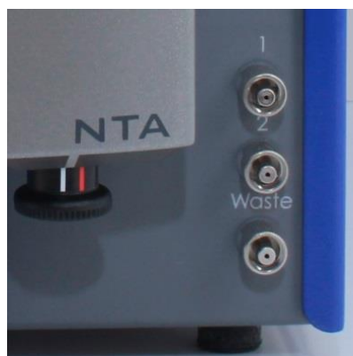
Figure 3-2: Fluidic connectors of the ZetaView® instrument located at the front side.
