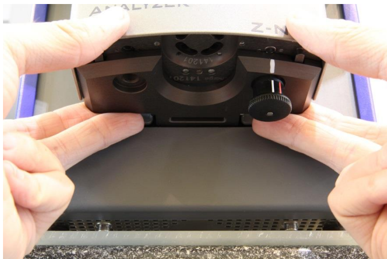
Figure 4-5: While locking the Cell assembly (white markings are in line with each other), hold the base plate at both sides with your fingers.
