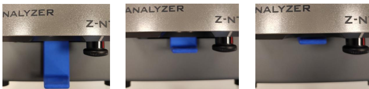
Figure 12-2: Positions of the manual fluorescence filter in scatter- (left) and in fluorescence mode (middle). Make sure not to push the filter to the top position (right), as this will block the microscope's beam path.
