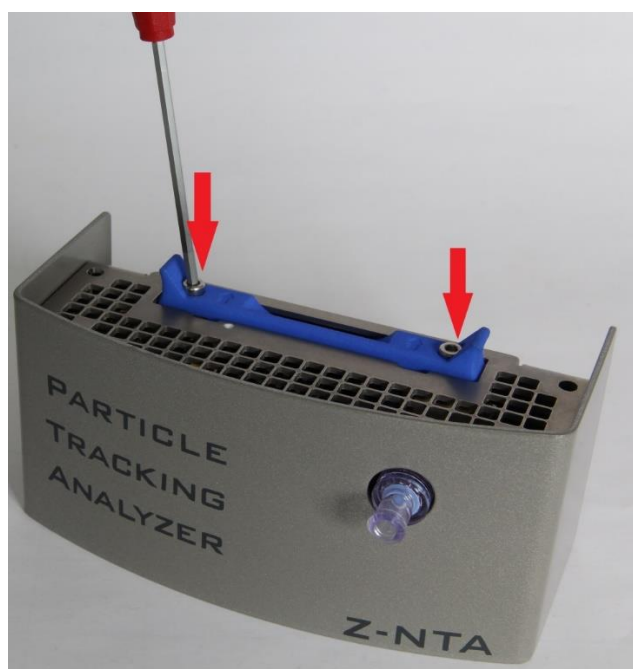
Figure 4-9: For removing the cell carrier, unscrew the screws on the left and right side.
