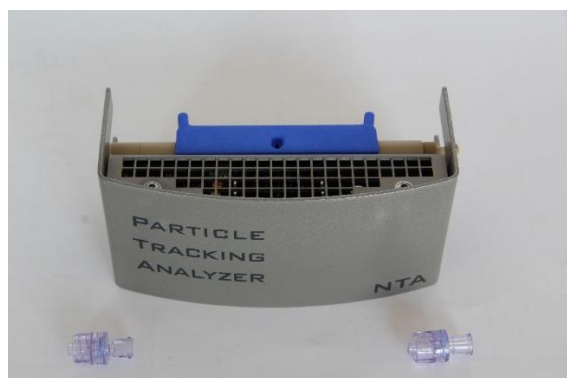
Figure 14-7: The left and right check valves must be unscrewed.
