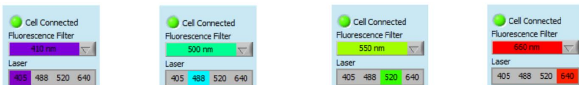
Figure 12-5: Laser wavelengths and corresponding fluorescence filters.
