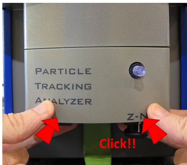
Figure 4-6: The Cell assembly clicks in when locking it on the ZetaView® instrument.
