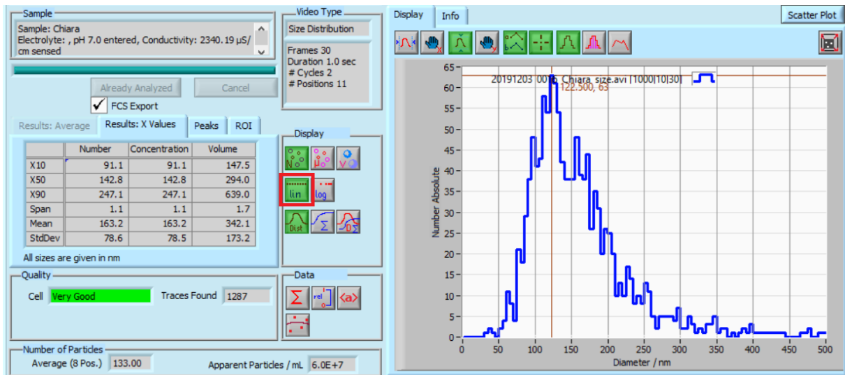
Figure 10-5: The histogram in a linear plot. The bin class “PSD nm / Class” was set to 5 here.
