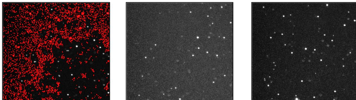
Figure 15-6: Examples of stray light patterns in a measuring cell filled with sample. Left: in the digital view. Middle and right: in the analog view with background of different intensity.
