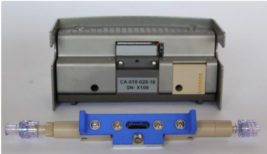
Figure 4-20: NTA Cell assembly shown from the back side. The cell has been removed.
