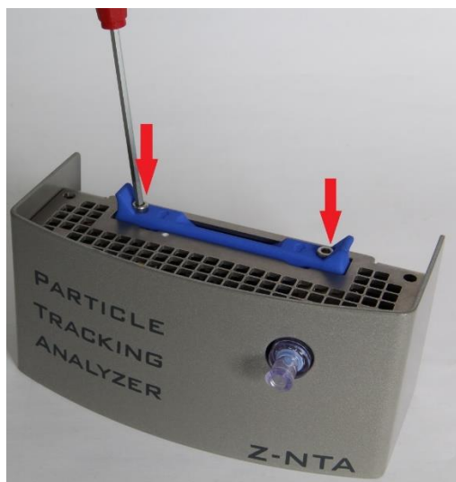
Figure 14-3: Remove both screws on top of the cell carrier.
